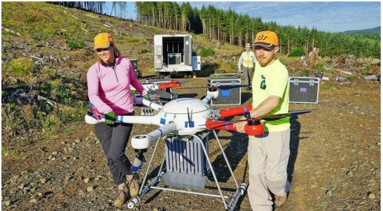
Figure 1: DroneSeed's new heavy duty tree seed planter. Can carry up to 300 seed pucks.
