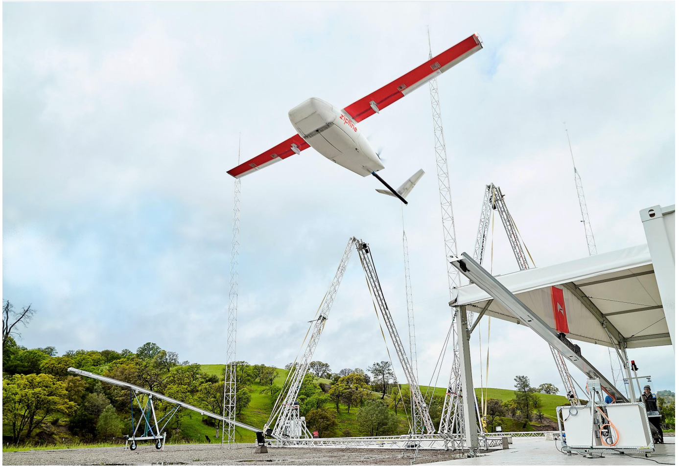
Figure 5: Zipline drones can go up to 50 miles per hour and travel a distance up to 100 miles.
